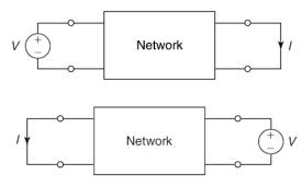
theorem, position of any passive element (R, L, C) do not change. Only the excitation and response are interchanged.
