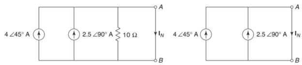
$$I_N = 4\angle 45^\circ + 2.5\angle 90^\circ = 6.03\angle 62.04^\circ \text{ A}$$
