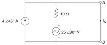
By source transformation, the network is redrawn as shown in Fig.
