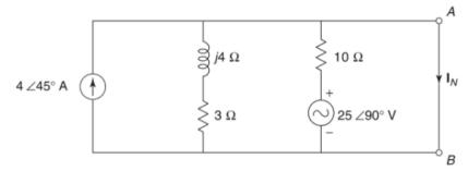
When a short circuit is placed across the  $(3+j4) \Omega$  impedance, it gets shorted
