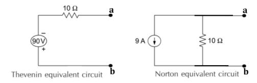
9) Determine the Norton's equivalent network across terminals A and B in the circuit
