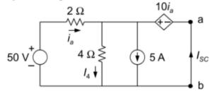
$$\frac{10i_a}{4} + 5 + \frac{10i_a - 50}{2} = 0 \quad \text{or} \quad 30i_a = 80 \quad \text{or} \quad i_a = 2.666 \text{ A}$$
