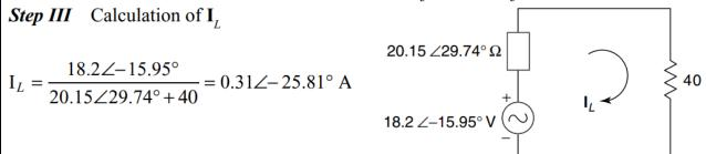
**15)** In the network shown in Fig., what load Z<sub>L</sub> will receive the maximum power. Also find maximum power.
