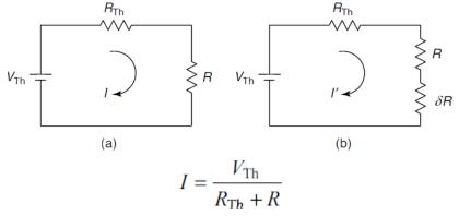
If the load resistance R be changed to  $R + \delta R$  as shown in Fig.(b) then the current flowing in the circuit is
