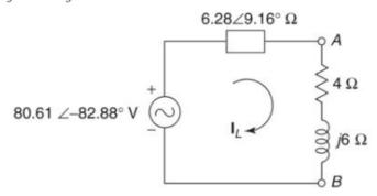
$$I_L = \frac{80.61\angle - 82.88^{\circ}}{6.28\angle 9.16^{\circ} + 4 + j6} = 6.52\angle - 117.34^{\circ} \text{ A}$$
