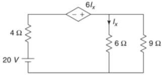
Step I Calculation of  $V_{\rm Th}$  Applying KVL to the mesh,
