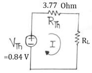
From maximum power transfer theorem,  $R_L$  = 3.77  $\Omega$
