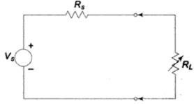
Current in the circuit is  $I = V_S/(R_S + R_L)$
