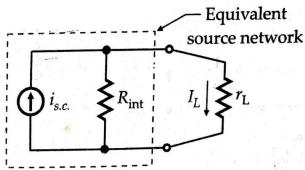
$\triangleright$  Reconnect the load resistor (RL) across the load terminals and the current through it (I<sub>L</sub>) is then given by
